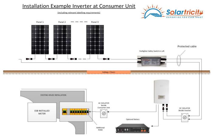
Above is a line drawing of a typical PV system. Your system may have one or two DC isolators, depending on whether the inverter is mounted downstairs or closer to the solar panels.
